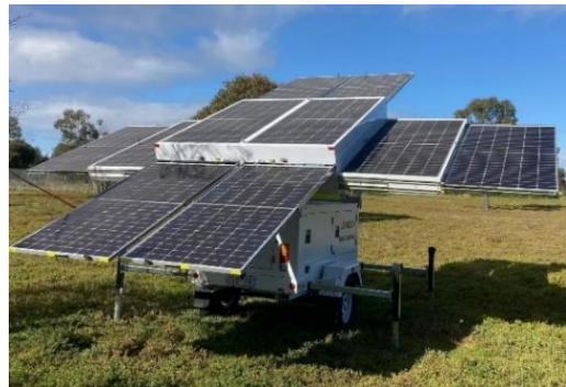
4.6kW Solar Array, 14kWh Battery Bank
