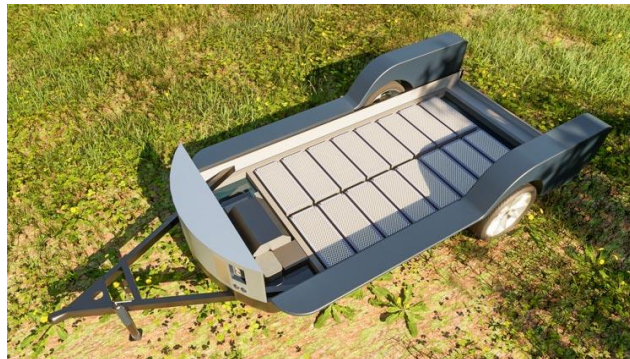
75kWh battery bank under floor of trailer
